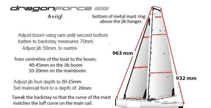
This should give you a good base setup for a correctly built rig.
